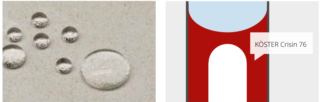
Hydrophobizing: Making the building material water repellent
